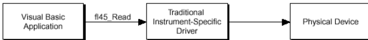
Figure 1. Although traditional instrument drivers manage low-level details for you, they restrict instrument interchangeability.
